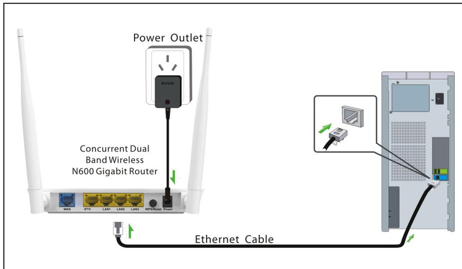
3. Connect the Ethernet cable from Internet side to the WAN port on the Router.
