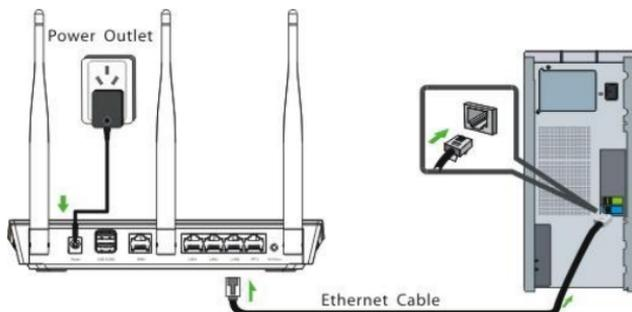
3. Connect the Ethernet cable from your ISP side to device's WAN port.
