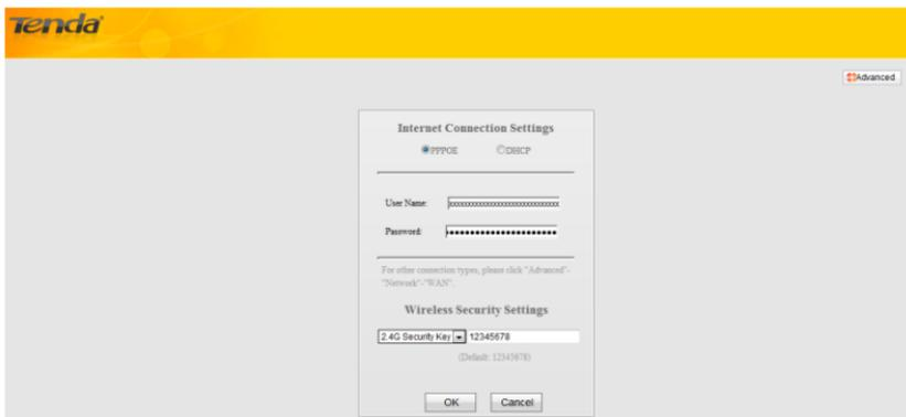
If you used to access Internet simply by connecting your PC directly to the modem with no need to configure any settings on your PC. Then select DHCP, enter a security key and then click OK.
