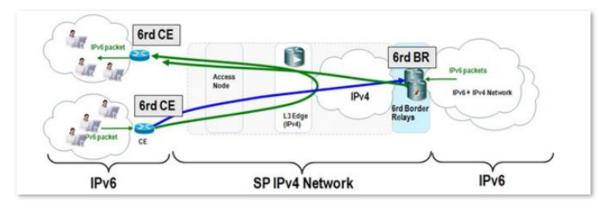
As shown in the figure above, the 6RD tunnel technology is used to implement mutual access between IPv6 islands, and the BR can also be used to access the IPv6 network after the BR.
