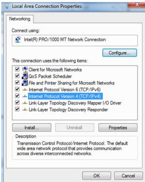
**Step 4** Select **Obtain an IP address automatically** and **Obtain DNS server address automatically**, and click **OK**.
