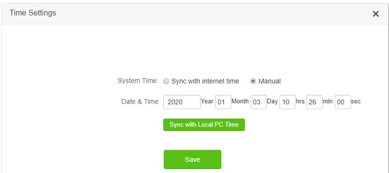
The screenshot shows the 'Time Settings' window with 'Manual' selected. The 'System Time' section has 'Sync with internet time' and 'Manual' (selected) radio buttons. Below, the 'Date & Time' section has input fields for Year (2020), Month (01), Day (03), hrs (10), min (26), and sec (00). There are two green buttons: 'Sync with Local PC Time' and 'Save'.
