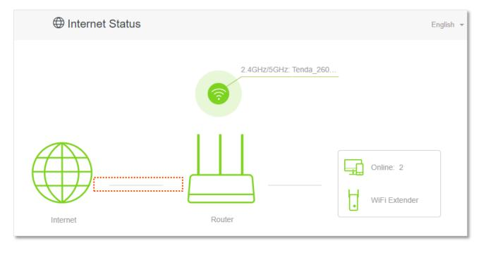
When a red cross and "Connection failed." are shown between the Internet and the Router, it indicates that the internet connection is abnormal. Please click Connection failed. to navigate to the Internet Settings page and follow the instructions to solve the problem.
