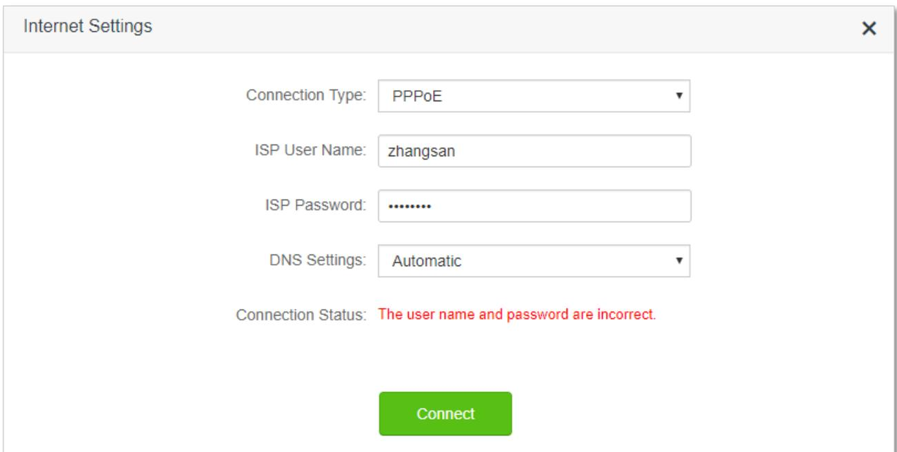
The screenshot shows a window titled "Internet Settings" with a close button (X) in the top right corner. Inside the window, there are four input fields: "Connection Type" set to "PPPoE", "ISP User Name" set to "zhangsan", "ISP Password" masked with seven dots, and "DNS Settings" set to "Automatic". Below these fields, the "Connection Status" is displayed in red text as "The user name and password are incorrect." At the bottom center of the window is a green "Connect" button.
