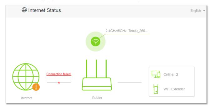
When "Please ensure that the cable between the Internet port of the router and the modem is properly connected" is shown on the page, ensure that the WAN port of the router and the LAN port of the modem or the Ethernet jack are connected properly. If the problem persists, contact the technical support for help.
