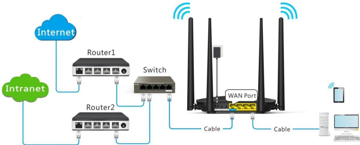
Router 1 accesses the internet and Router 2 the intranet. AC5 gets IP address to access the internet from Router 1 automatically. Set static route on AC5, achieving LAN clients access both internet and intranet.
