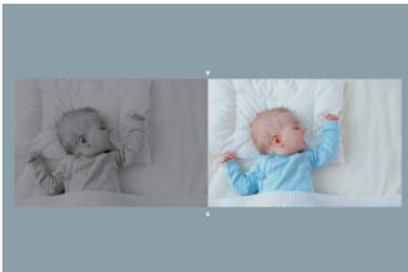
Equipped with high sensitive image sensors, CP6 shows the color of delicate image even in low-light condition. The four built-in 850 nm infrared lights adopt enhanced night vision algorithm, producing clearer night vision and increasing the distance of night vision up to 12 m(40ft) .
