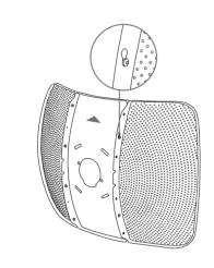
6 Insert the CPE into the CPE seat from the front side of the center
