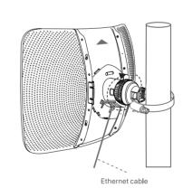
To prevent the deformation of the reflector panels and decreasing of bridging quality, DO NOT face the reflector panels down and put them on a desk or a horizontal plane while and after fixing the CPE seat.
