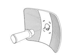
3 Remove the Ethernet port cover from the CPE seat. Align the slots of the CPE seat with the abutted edges of the center reflector panel and side reflector panels, and four hooks of the CPE seat with the four slots of the center reflector
