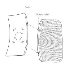
5 Fix the reflector panels with the included screws
