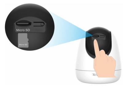
**Step 2** Log in to TDSEE App to check whether the Micro SD card can be identified normally.
