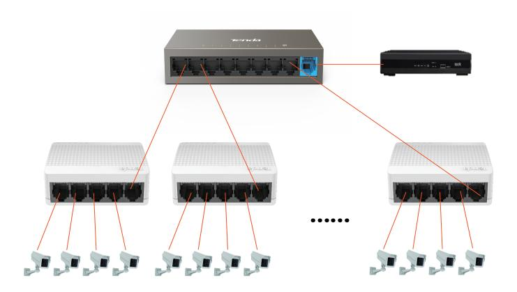
Connect 8 S105 to RJ45 ports of TEF1109DT, and a NVR to its uplink port. Then you can connect up to 32 IP cameras for network.
