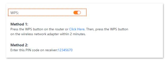
Press the **WPS** button on the modem router for 3 seconds and then release it, or click **Click Here** under **Method 1** on the web UI. The **WPS** LED indicator starts blinking, indicating the devices are negotiating.
